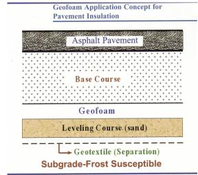
The depth requirements for pipeline burials below frost penetration could be reduced if geofoam is used.<sup>14</sup>
