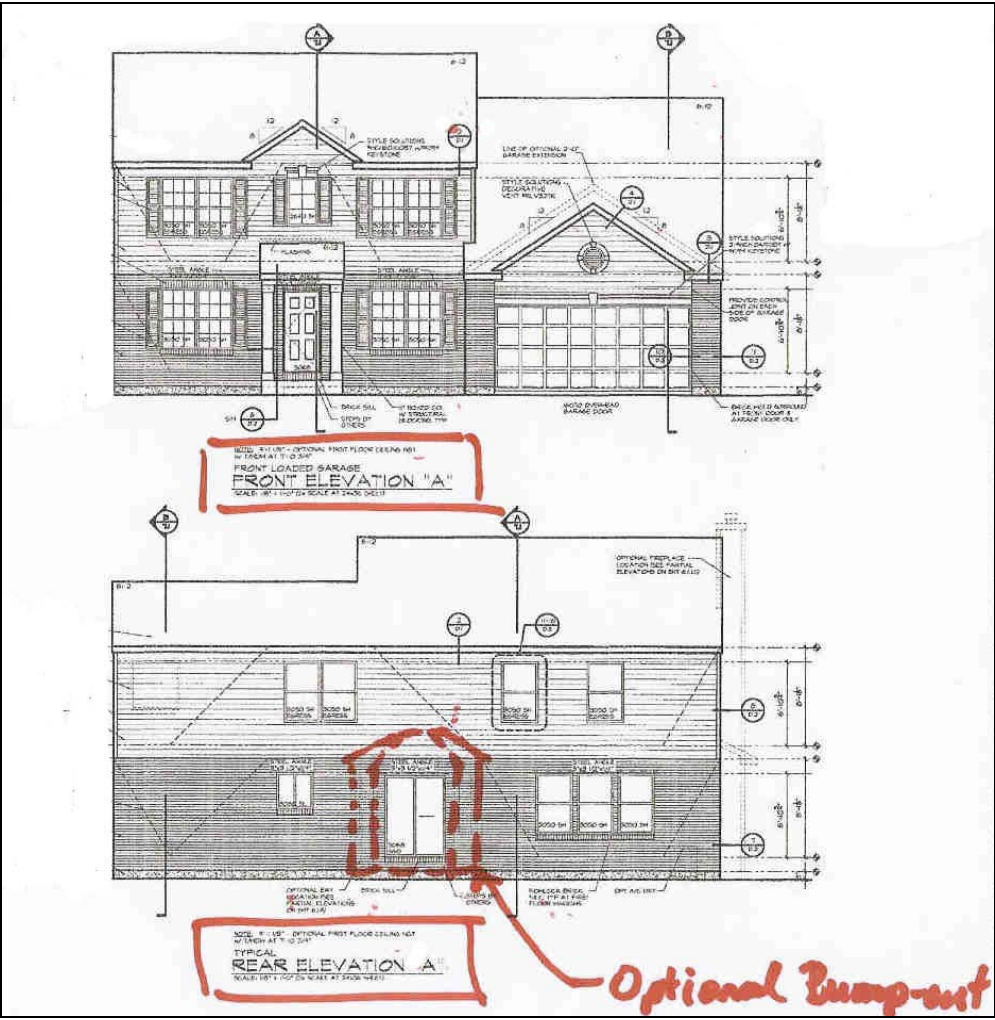
Figure 3: Plan Elevations Showing Front and Rear Braced Wall Line Conditions and Optional Plan Features.
